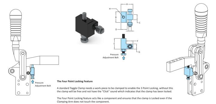
The user can increase or decrease the force required to finish the Toggle Action by adjusting the Screw.
